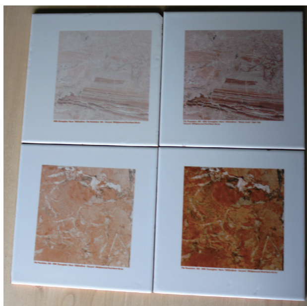
Fig. 9 Samples printed on ceramics with a Konica Minolta inkjet print head (Note 1).
